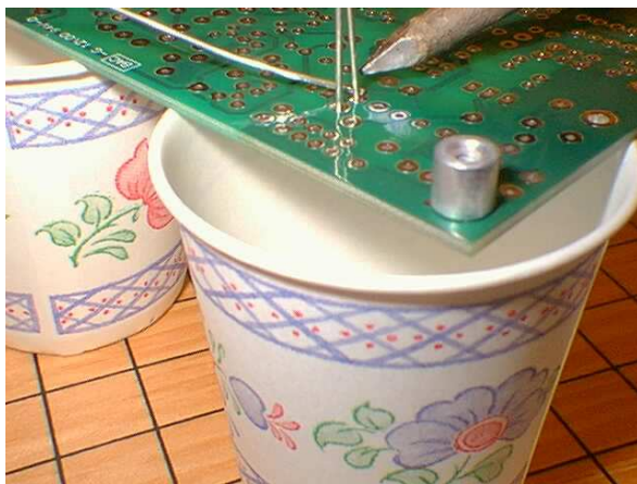
D13 being soldered.
